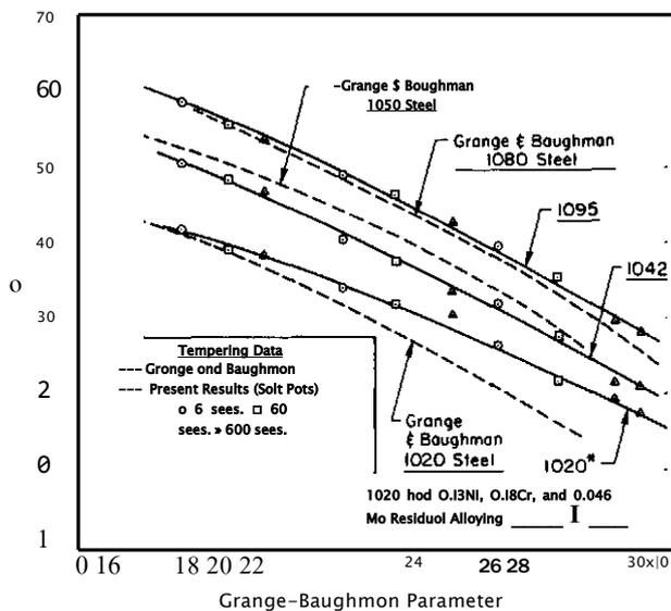
Fig. 1—Comparison of tempering data for carbon steels from present investigation ("salt pots") and those obtained by Grange and Baughman.<sup>7</sup> The present results are for isothermal treatments lasting 6, 60, or >600 seconds.
