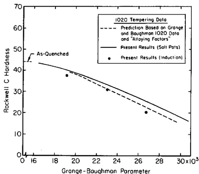
Fig. 6—Comparison of present 1020 tempering data from salt-pot and induction treatments, with a prediction based on Grange and Baughman's 1020 results and hardness-increment factors ("alloying factors").
