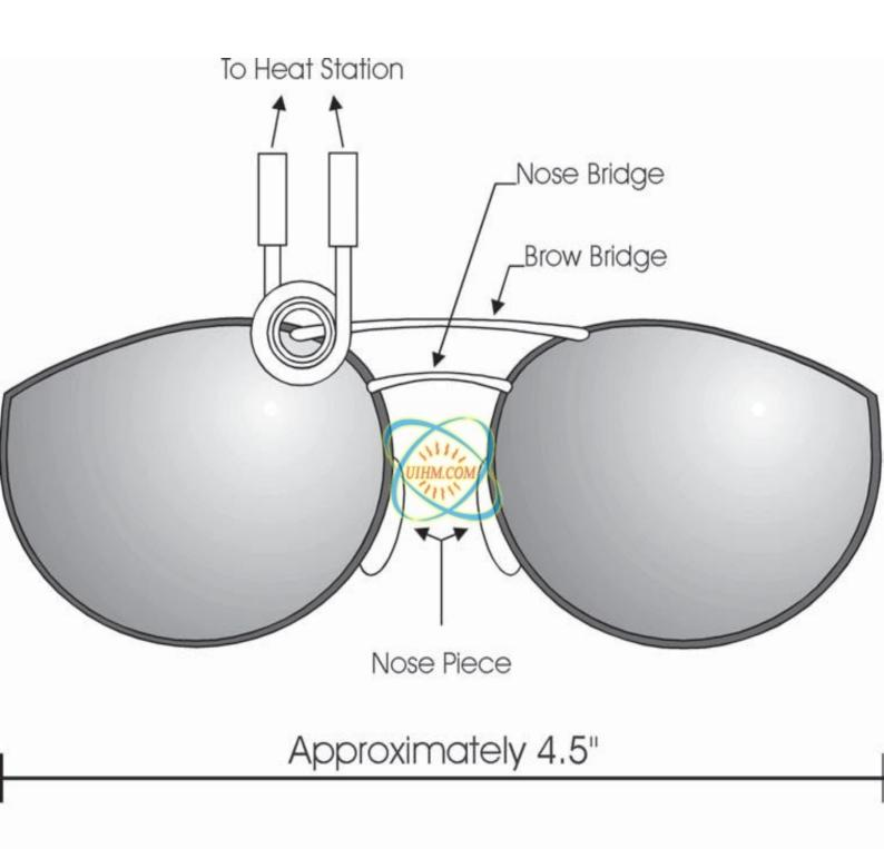
Note: Frame Is Brazed Prior To Assembly Of Lenses.
