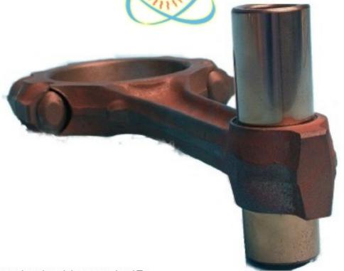
Final assembly of wrist pin & rod
