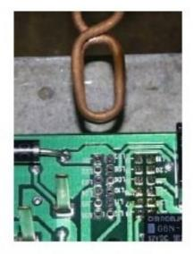
Twelve preforms in place for soldering
