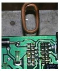
Completed soldering of the 12 post service@uihm.com
